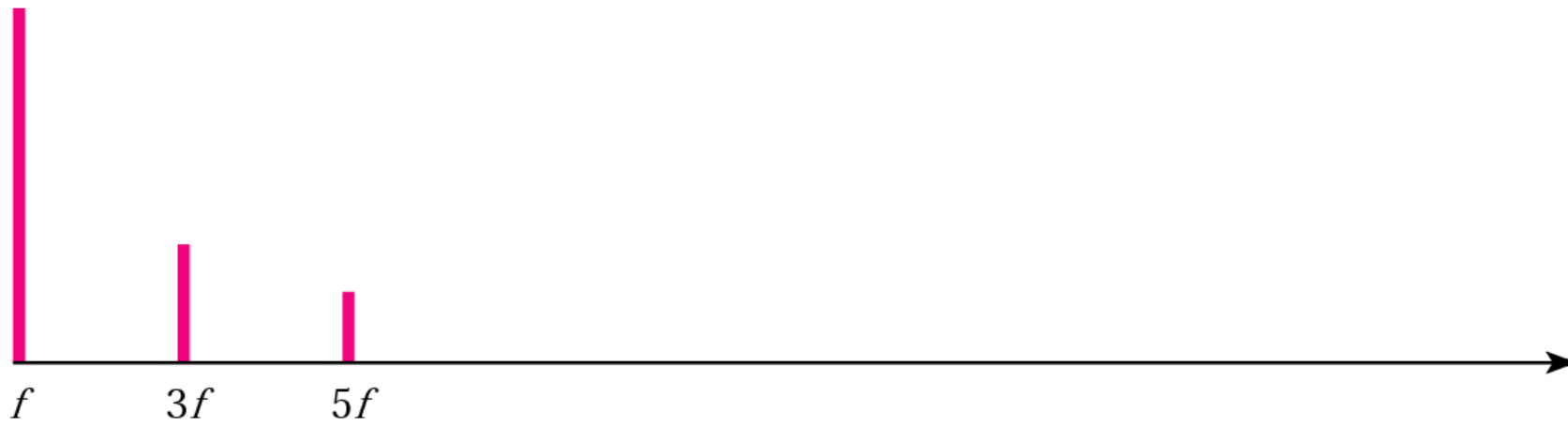
b. Frequency spectrum of an approximation with only three harmonics
